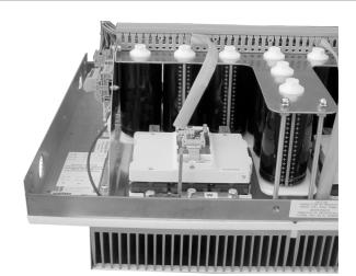
Modular SEMISTACK® using SKiiP® 3 to give 1/6th of a 4-Quadrant Converter (700 kW, 660 Arms) for wind generators up to 2 MW
